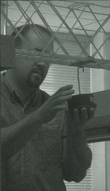
ABOVE: Physics professor Dr. Lawrence adds weight to a bridge to see how much weight it will hold without breaking.
